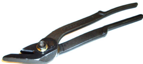
Model : OV-BSC-25 Type : Side Action Type Cutter Strap Width : 13mm (1/2") to 25mm (1") Strap Thickness : 0.4mm(0.015") to 0.7mm(0.027")
