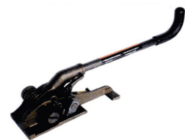
Model : OV-BT-32 Type : Windlass Type Tensioner Strap Width : 19.0mm(3/4") to 32.0mm(1 1/4") Strap Thickness : 0.6mm(0.023") to 1.2mm(0.047")
