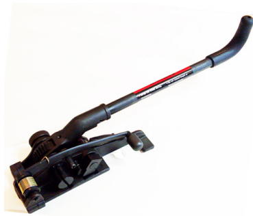
Model : OV-BTC-32 Type : Windlass Type Tensioner with Cutter Strap Width : 19.0mm(3/4") to 32.0mm(1 1/4") Strap Thickness : 0.6mm(0.023") to 1.2mm(0.047")
