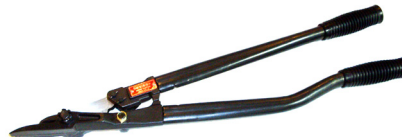
Model : OV-BSC-50 Type : Side Action Type Cutter Strap Width : 13mm (1/2") to 50mm (2") Strap Thickness : 0.4mm(0.015") to 1.0mm(0.040")
